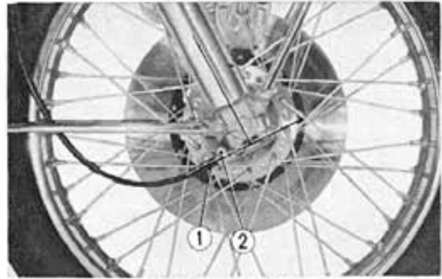
Fig. 13-13 ① Speedometer cable ② Setting screw
