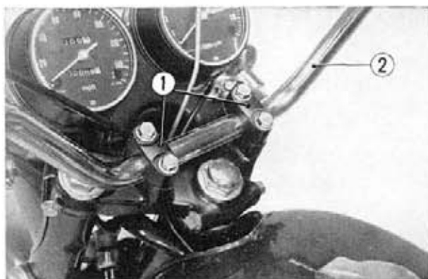
Fig. 11-3 ① Upper handle holders ② Handle bar
