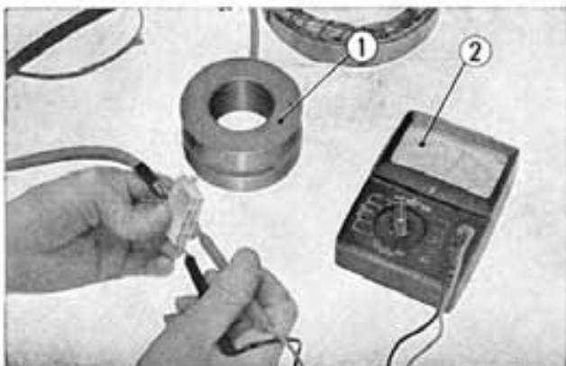
Fig. 8-8 ① Field coil ② Tester
