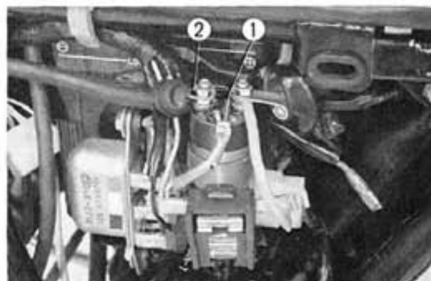
Fig. 9-3 ① Magnetic switch ② Starting motor cable
